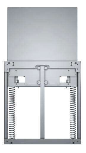
The WallLift-02 is the perfect solution to move your touchscreen up and down. It offers a partially overlapping weight range giving the installer the choice between a travel of 400mm and 650mm. With a weight capacity of up to 90kg, the iBT WallLift-02 offers a compact and stylish stainless steel design that is hidden behind the touchscreen.
